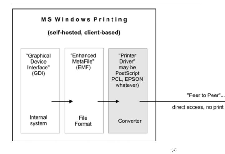
Figure 19.1: Windows Printing to a local Printer
