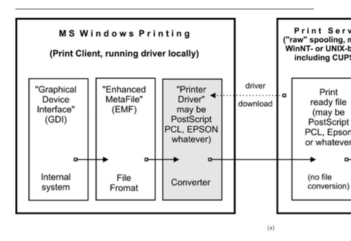
Figure 19.11: Print Driver execution on the Client
