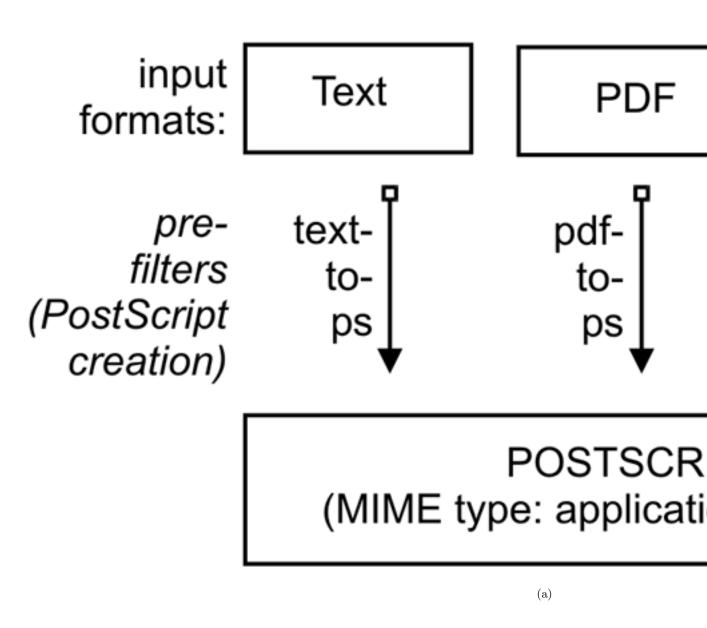
Figure 19.4: Prefiltering in CUPS to form Postscript
